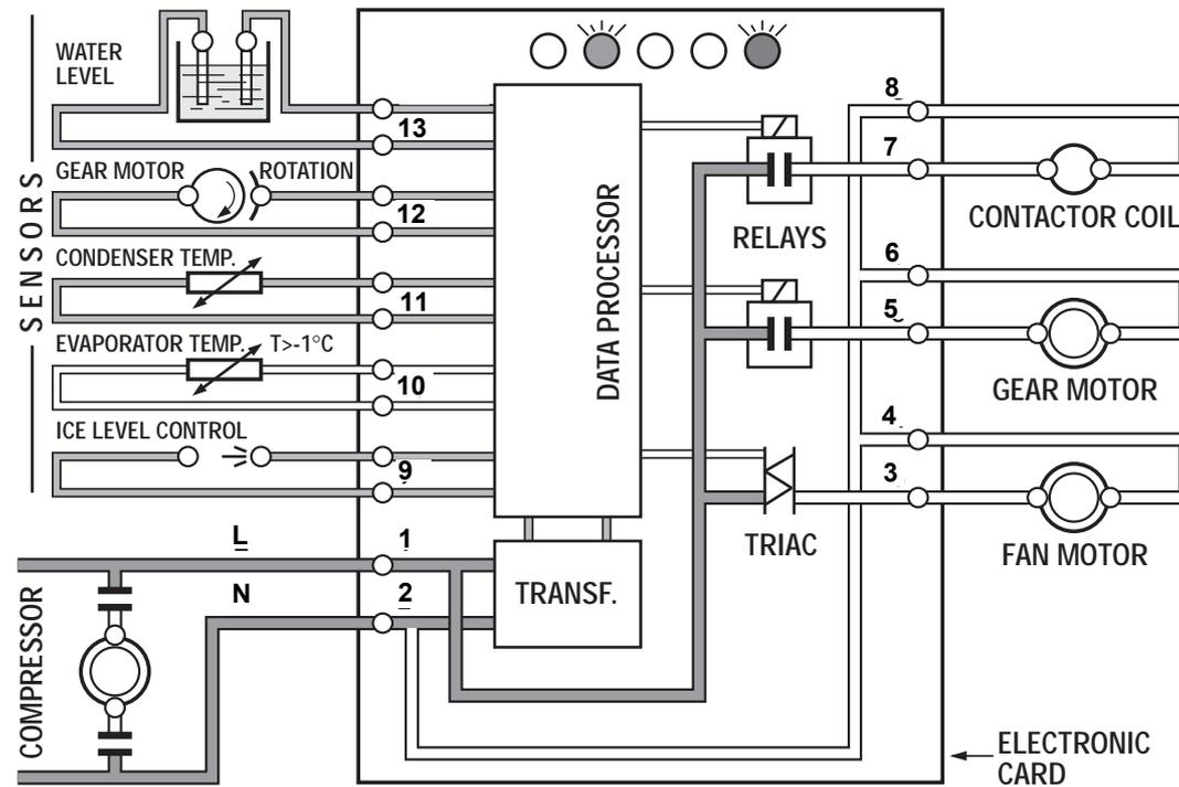
This will cause a gradual decrease of the water level in the float reservoir and as soon as the level gets below the two vertical metal pins, the flaker stops to operate (compressor first and 3' later the gear reducer) and the **YELLOW warning LED** will glow to signal the shortage of water (Fig. 4)
