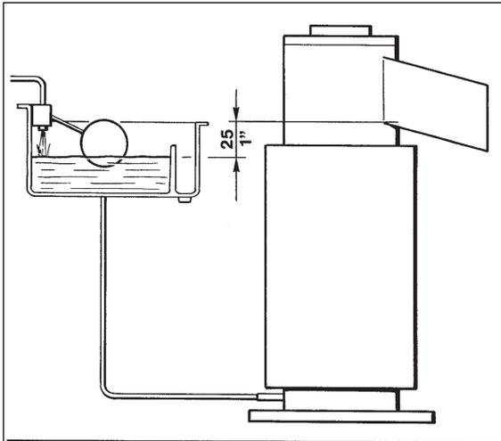
When the water level is above or below the correct one, adjustment can be performed by raising or lowering at the measure required, the water reservoir and its mounting bracket.
